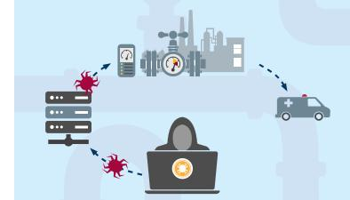
**HISTORICAL EXAMPLE:** In 2017, an actor installed malware on safety instrumented systems (SIS) at a petrochemical facility in Saudi Arabia in an attempt to cause damage and injuries. A lack of isolation of the critical SIS from the ICS network likely contributed to the compromise.
