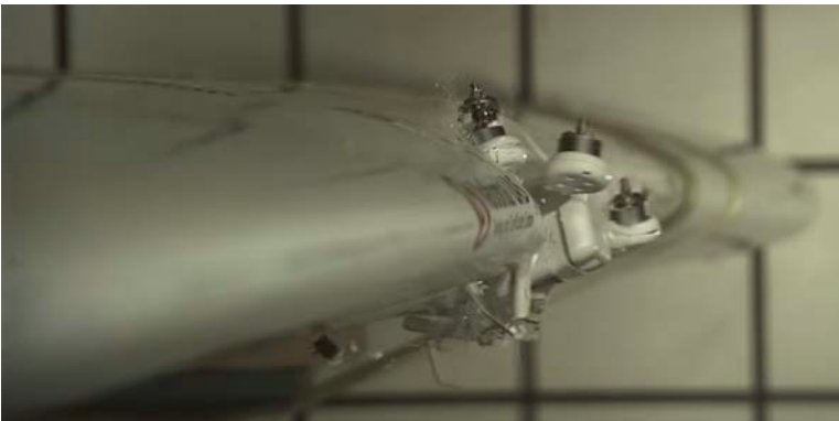
Experiment; Drone Striking a Wing
